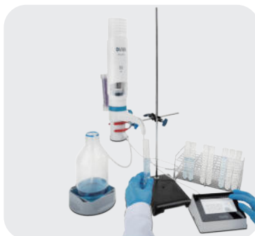
Manual free dispensing: Manually control aspiration and dispensing volumes.
