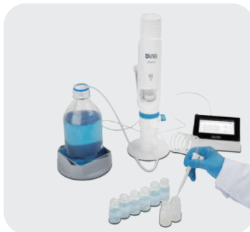
Automatic fixed-volume dispensing: Set dispensing interval, volume, and repetitions; manually trigger the first dispense, then the program continues dispensing according to the set interval.
